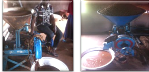
Figure 4. Photos of improved “spinning” roaster (top) and photos of mill used typically for grinding corn for staple foods grinding shea kernels into paste after being roasted (bottom). Taken by the author during field study (August 2014).
